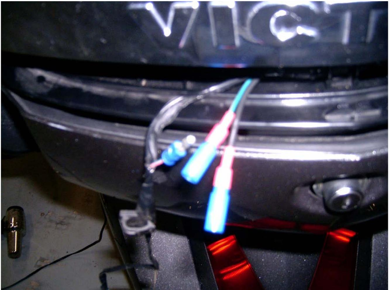
I removed the top panel behind the right speaker grill so that I could run my new wire through the original wire loom down through the hinge.
