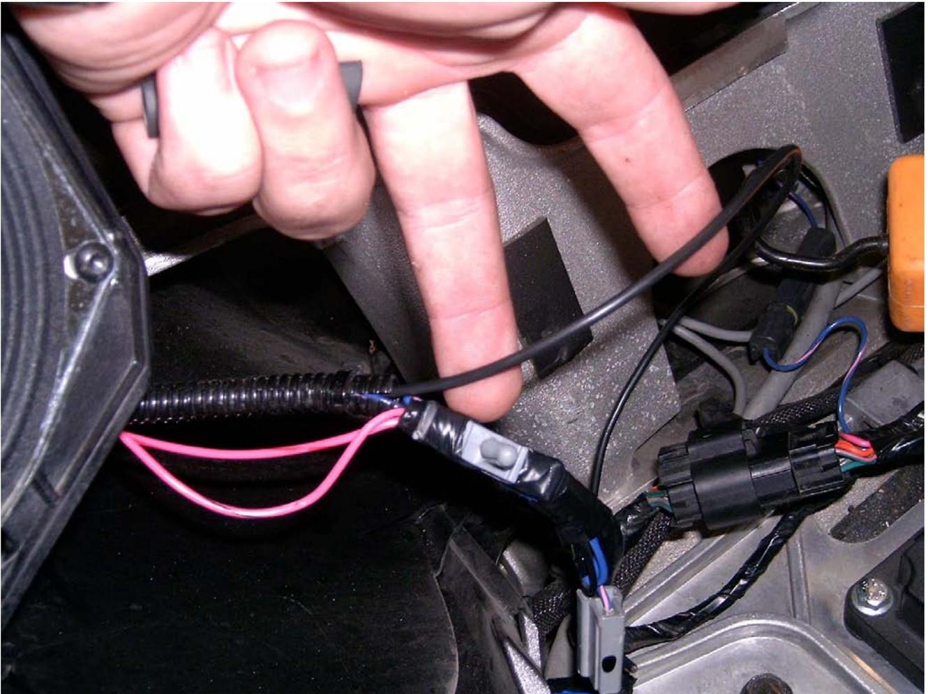
I used 3 tap splices to tap into the turn signals and brake and ran 3 wires over to the controller and connected them there using the scotch locks that came with the kit. I did this because I did not want my factory lights to change only wanted the trunk lights to change.
