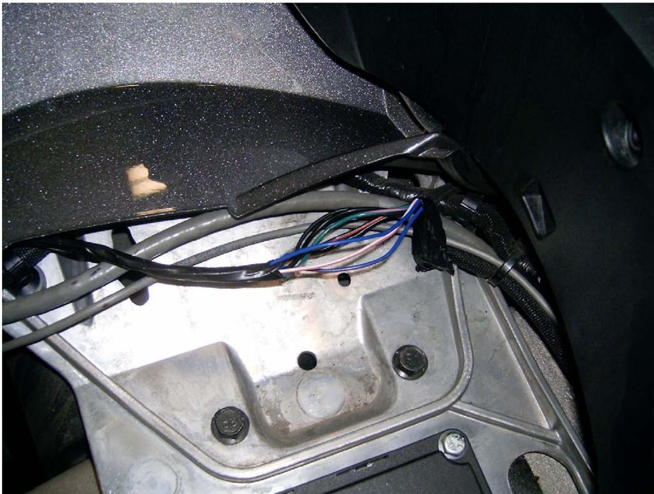
Here is where I ran my new wire from after removing the tape. Note that the wire is between the top of the lid and the outside of it.
