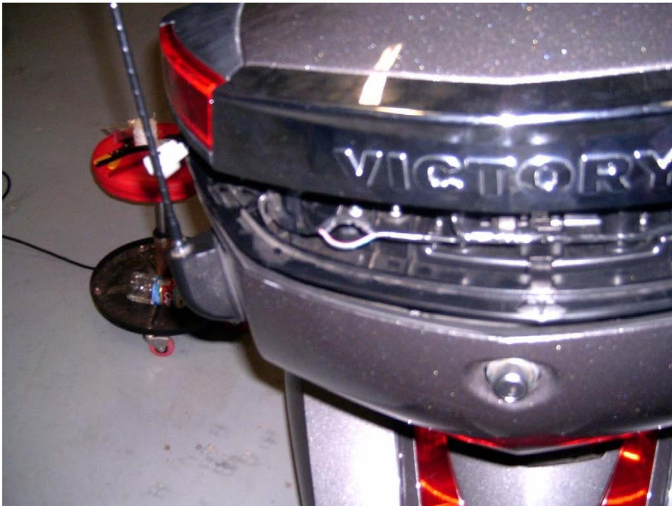
Once I cut the green/pink wire going to the left light I put a male connector on the side going to the light and female connector on both the new wire and the end of the old wire so that I could return it to factory if I need to.
